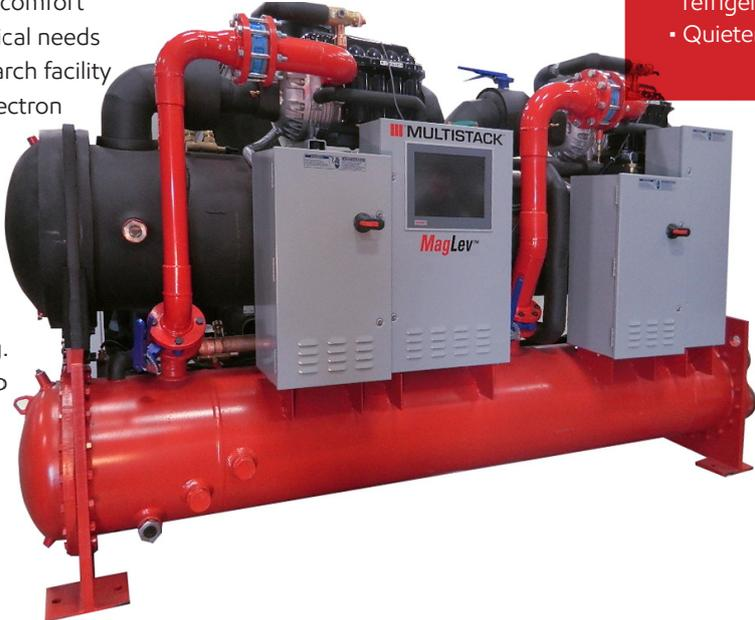
A Multistack chiller with MagLev® centrifugal compressors provides 300 tons of cooling capacity. MagLev compressors use leading-edge technology with oil-free, magnetic levitation bearings.
