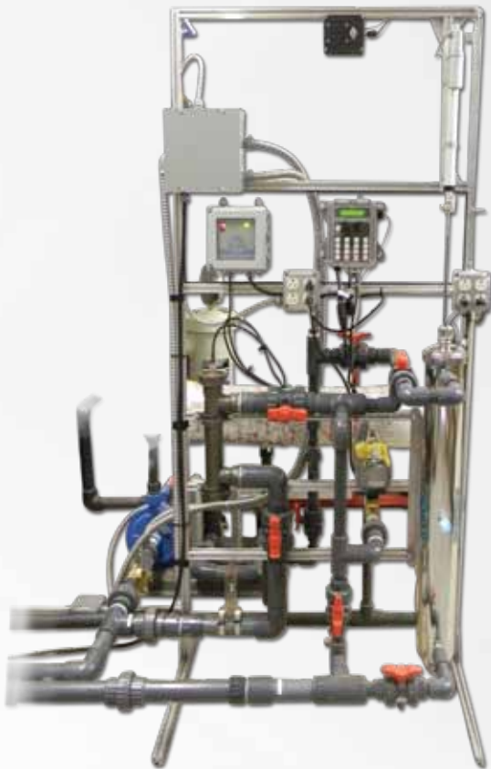
The eH 2 O non-chemical water treatment system including Tri-Tron pulse-powered mineral precipitation device, sanitron ultraviolet purified with automatic cleaning, and Microtron conductivity controller.
